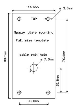
If the spacer plate is used the reader cable may be brought out of one of four exit points on the spacer: top, bottom, left or right. This enables the cable to be run on the surface of the wall. If no spacer plate is used a recommended hole size of 7.5 mm must be drilled in the wall at the cable exit position to allow the cable to exit perpendicular to the reader.
