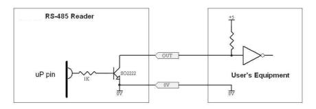
Schematic of Output, showing connection to TTL device
